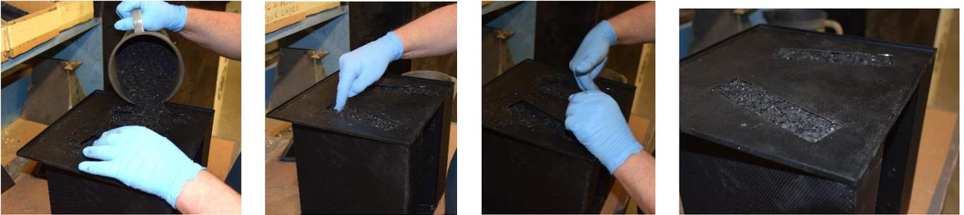
**Note:** You are sure that the charcoal is well packed inside the filter when you can't see the light passing through the metal container.
