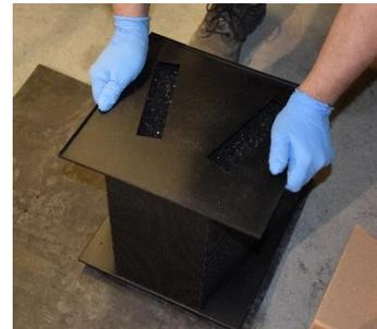
5. It is very important to fill completely the canister up to the edge. You can use your fingers to push the charcoal each sides of the openings. Replace the black door with the two screws.
